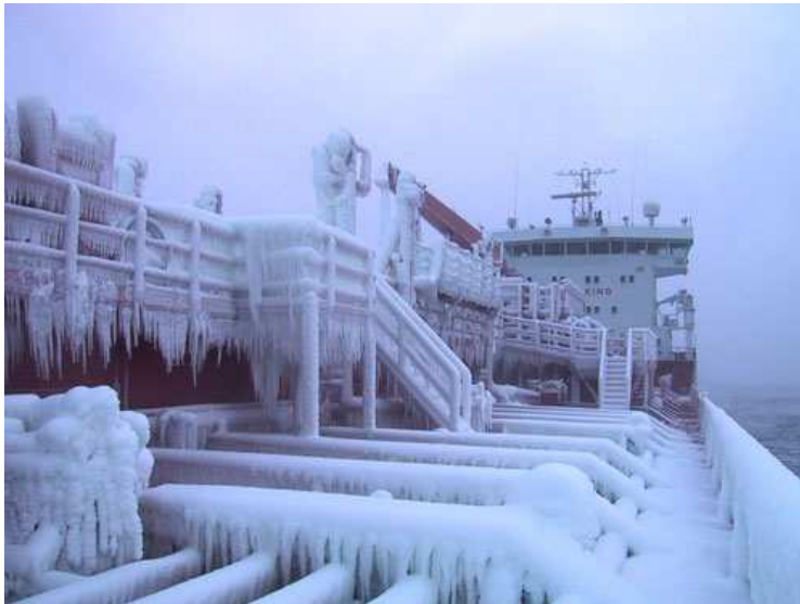
Icing of deck space and cargo structures (Eknes, 2004)
