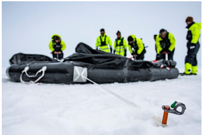
09h56 LT: Lashing the Polar Shelter' strap into the ice & Inflating of the 1 st Polar Shelter
